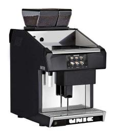
602620 (UTANGOACE1SELFLC) Full-automatic machine, 1 group, 220x40 ml espresso cup/hr, 6,5 liter steam/coffee boiler, 1x1,7 kg and 1x1,2 kg coffee hopper, programmable water, Cappuccinatore device for hot milk and foam drinks
